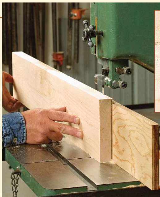
Now push gently and let the blade do the work. Pushing too hard will make the blade flex sideways, which will cause it both to overheat and to drift off line. With the blade, fence, and guides properly aligned and adjusted, the back of the blade should be centered in its kerf (inset).
