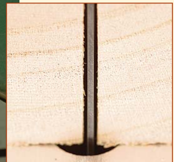
Now push gently and let the blade do the work. Pushing too hard will make the blade flex sideways, which will cause it both to overheat and to drift off line. With the blade, fence, and guides properly aligned and adjusted, the back of the blade should be centered in its kerf (inset).
